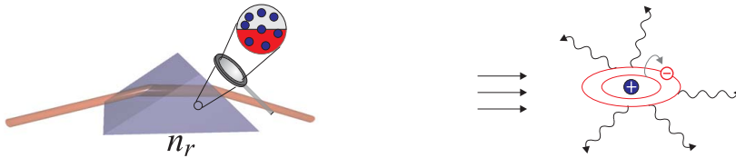
Figure 8.6: (Left) Macroscopic refraction and (right) microscopic scattering. See also (watch talk) .
